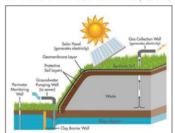
A cross-section of the environmental protection systems and solar panels that the Materials Innovation and Recycling Authority has installed at the Hartford landfill.
